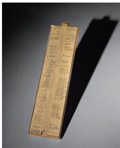
Figure 14. A Wollaston equivalent scale from 1820 with German labeling, from the collection of the Deutsches Museums in Munich.
